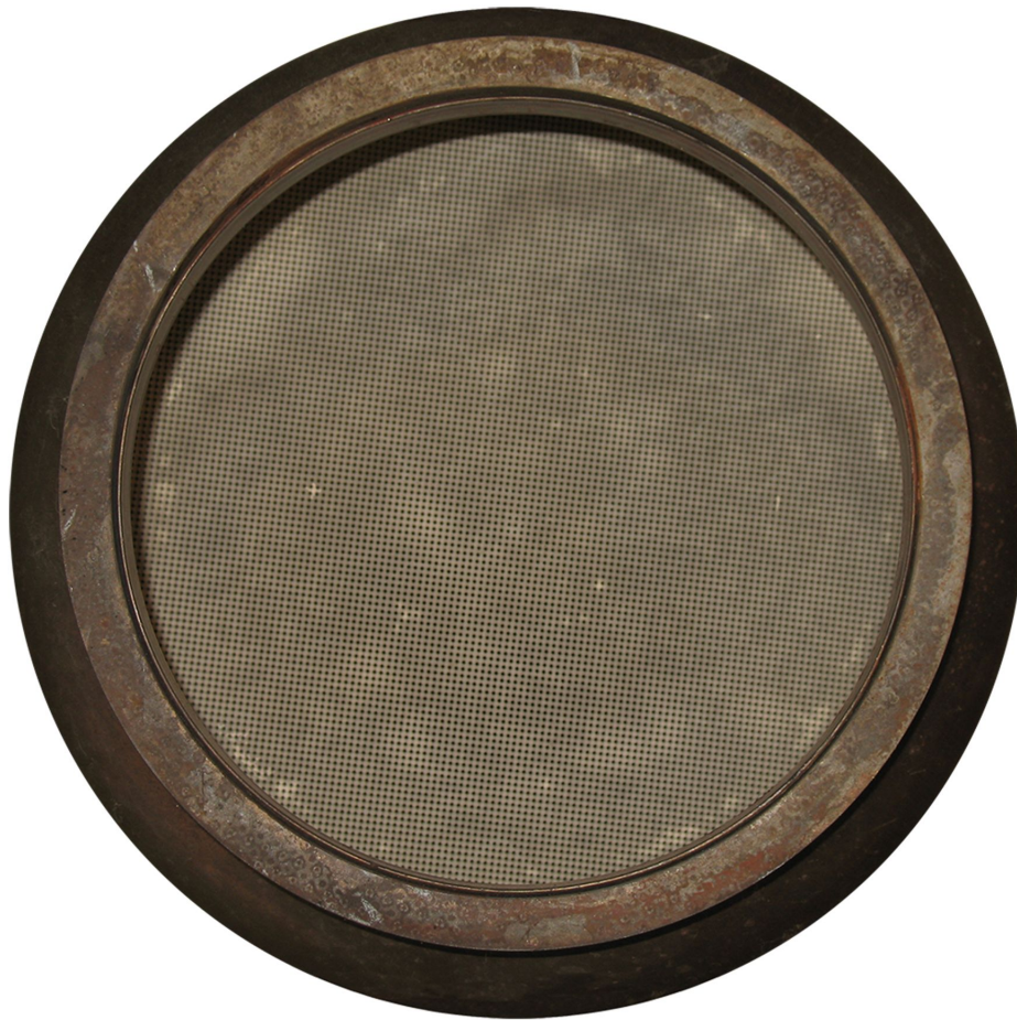
Figure 35 Diesel Particulate Filter (DPF) Inlet – Clean.
