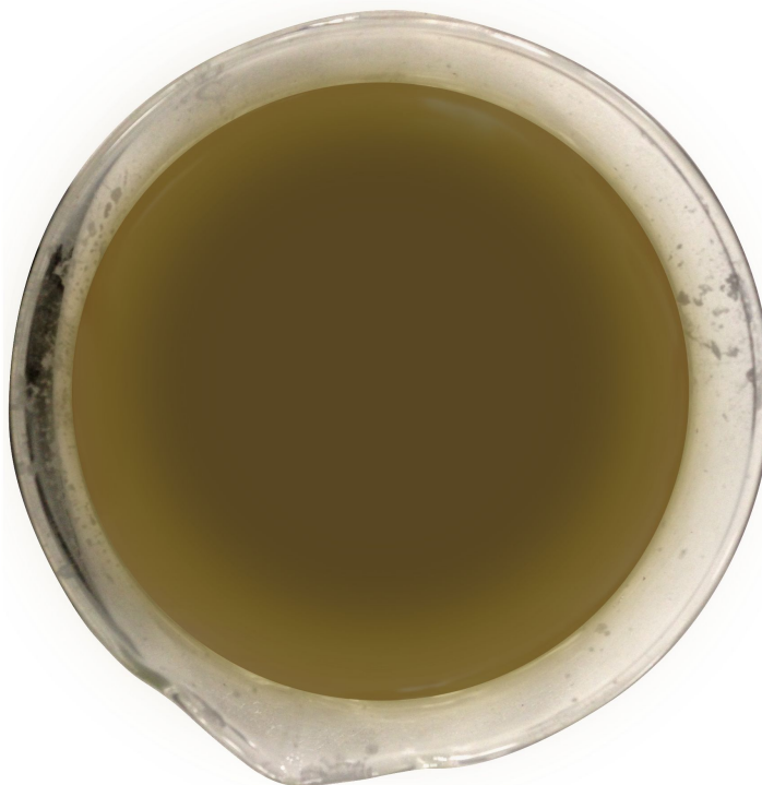
Figure 56 Heavily Contaminated DEF.
