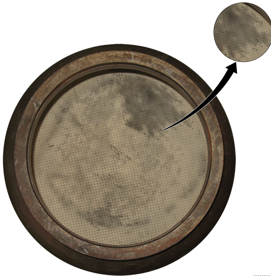
Figure 43 Diesel Particulate Filter (DPF) Outlet – Coolant Staining.
