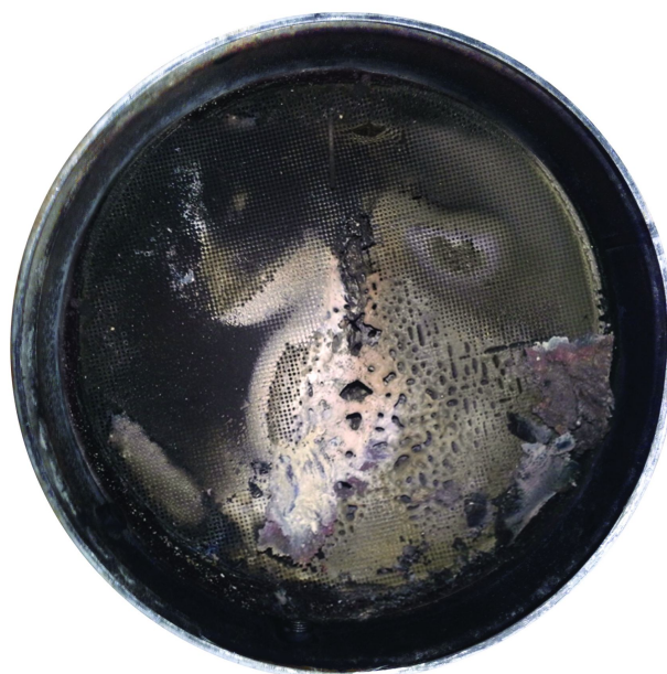
Figure 17 DOC Inlet / Outlet Face Excessive Oil or Fuel.
