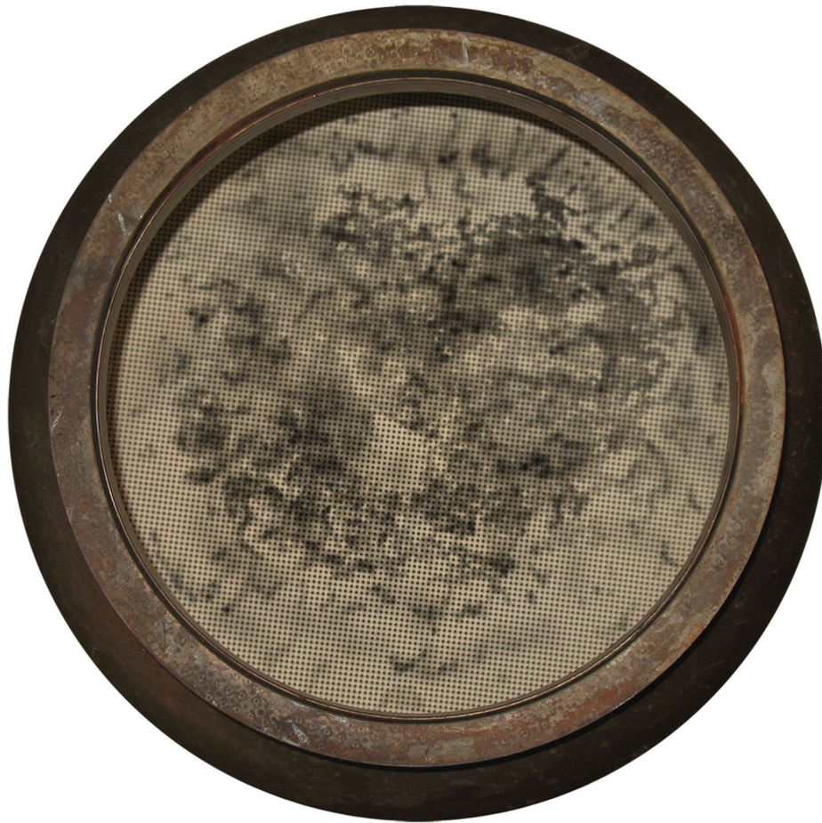
Figure 41 Diesel Particulate Filter (DPF) Outlet – Excessive Soot Stains.
