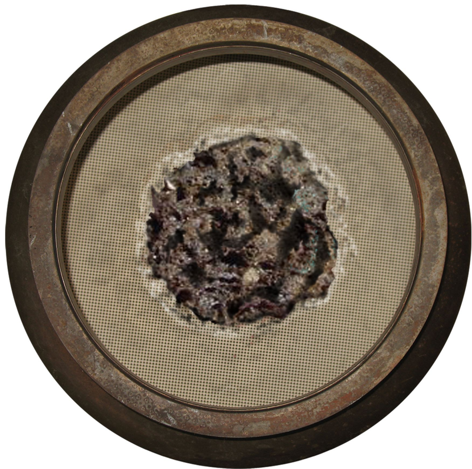
Figure 44 Diesel Particulate Filter (DPF) Outlet – Melted.
