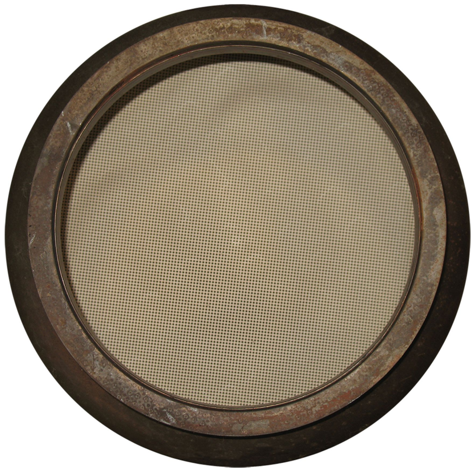
Figure 32 Diesel Particulate Filter (DPF) Inlet – New.
