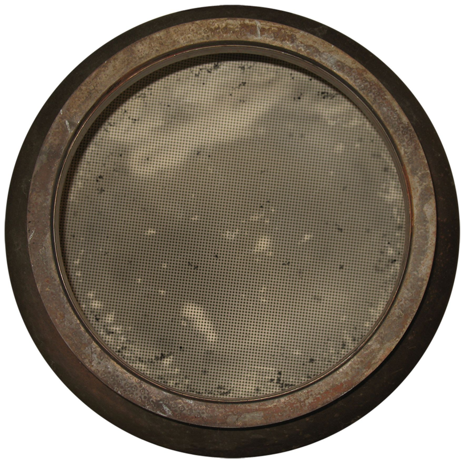
Figure 34 Diesel Particulate Filter (DPF) Inlet – Dirty and Usable (2).
