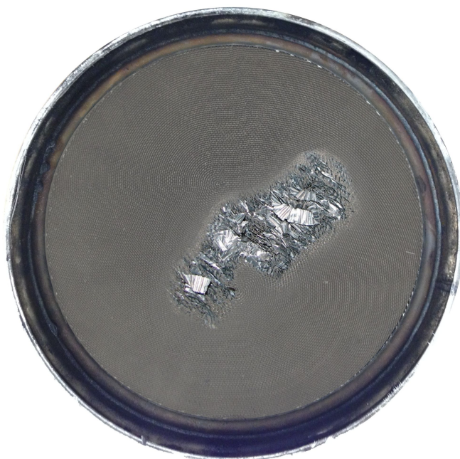
Figure 18 DOC Inlet / Outlet Face Gouge.
