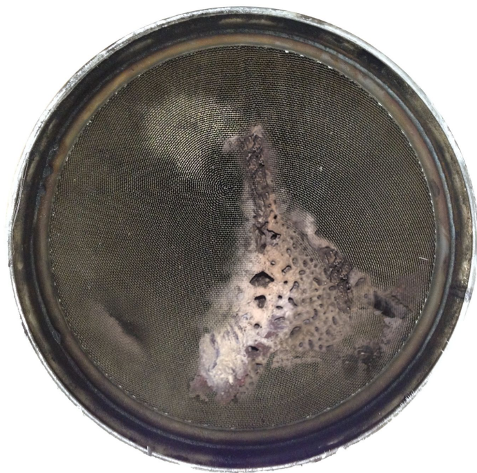
Figure 30 Diesel Oxidation Catalyst (DOC) Inlet / Outlet – Melted.
