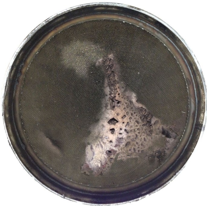
Figure 30 Diesel Oxidation Catalyst (DOC) Inlet / Outlet – Melted.
