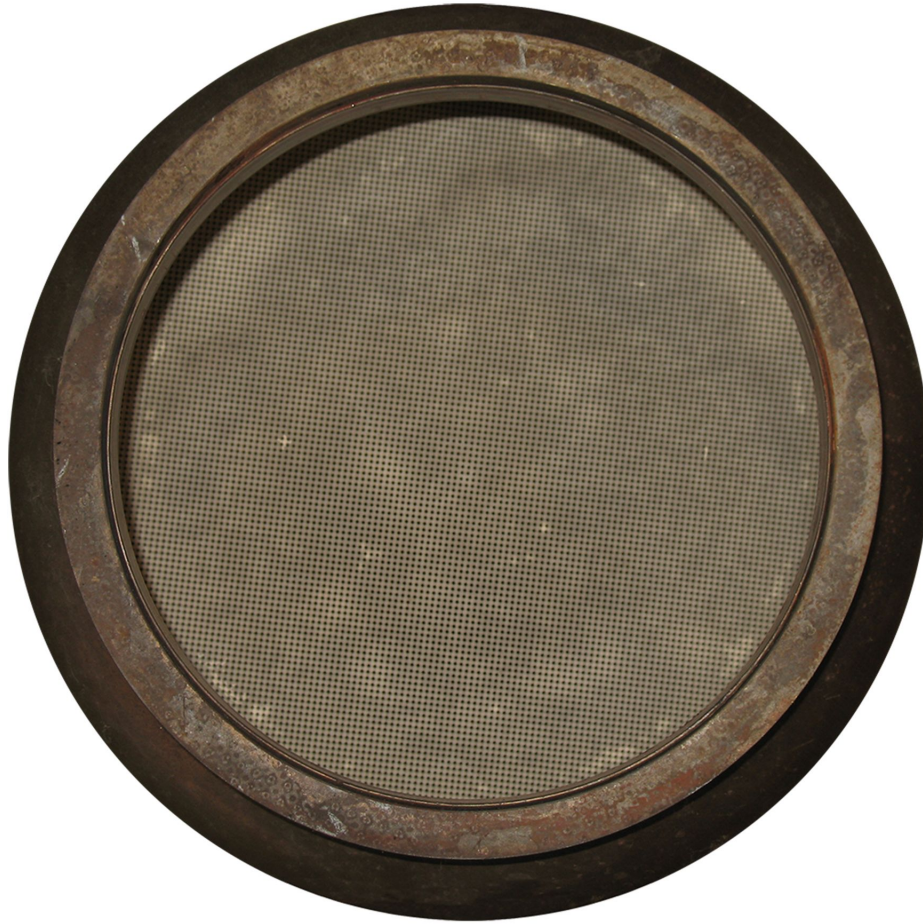
Figure 35 Diesel Particulate Filter (DPF) Inlet – Clean.
