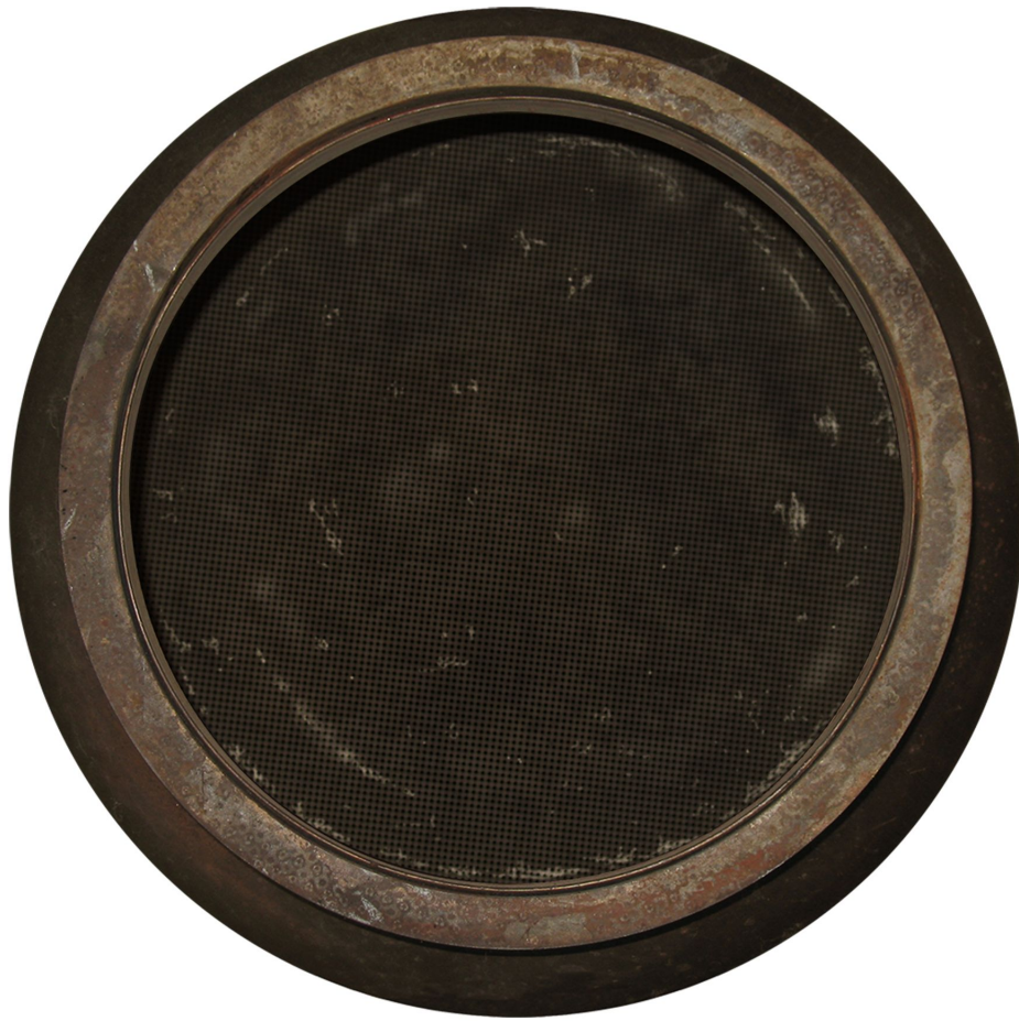
Figure 33 Diesel Particulate Filter (DPF) Inlet – Dirty and Usable (1).
