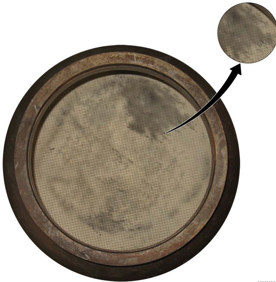
Figure 43 Diesel Particulate Filter (DPF) Outlet – Coolant Staining.
