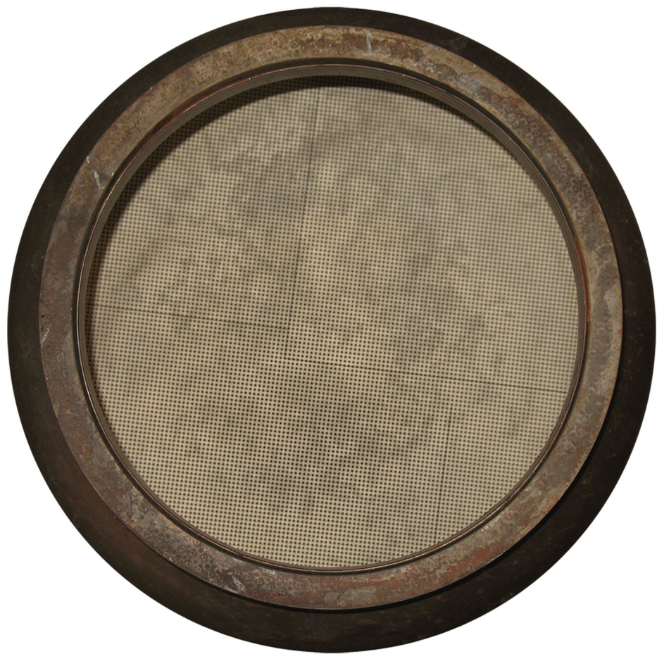
Figure 42 Diesel Particulate Filter (DPF) Outlet – Face Cracked.
