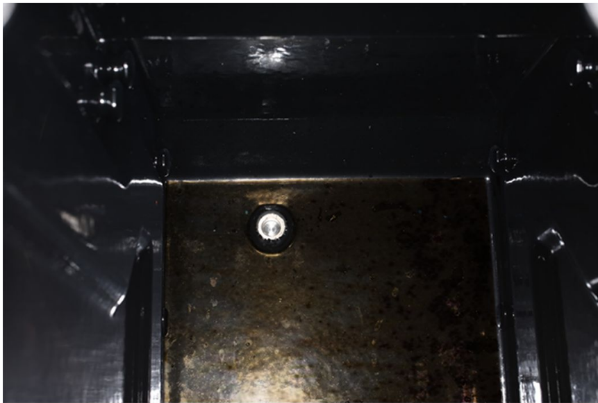
Figure 55 Debris on Bottom of DEF Tank.
