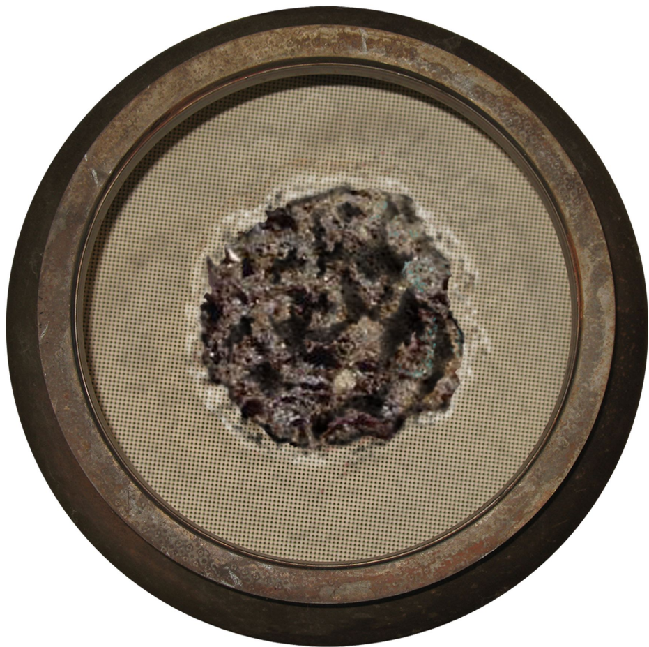
Figure 44 Diesel Particulate Filter (DPF) Outlet – Melted.
