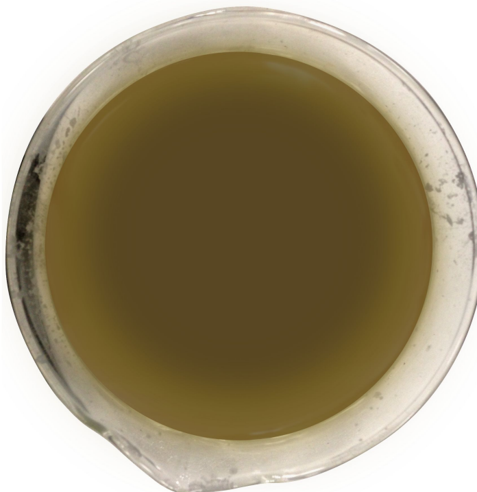
Figure 56 Heavily Contaminated DEF.
