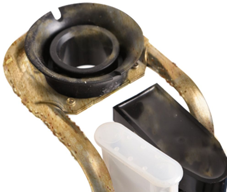
Figure 54 Oily Substance On The Def Tank Pickup Assembly.
