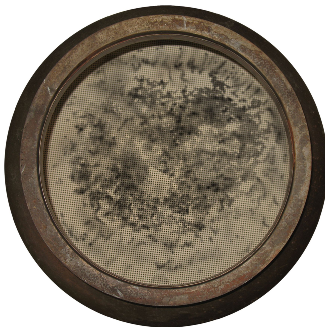
Figure 14 DPF Inlet / Outlet Face Excessive Oil or Fuel.
