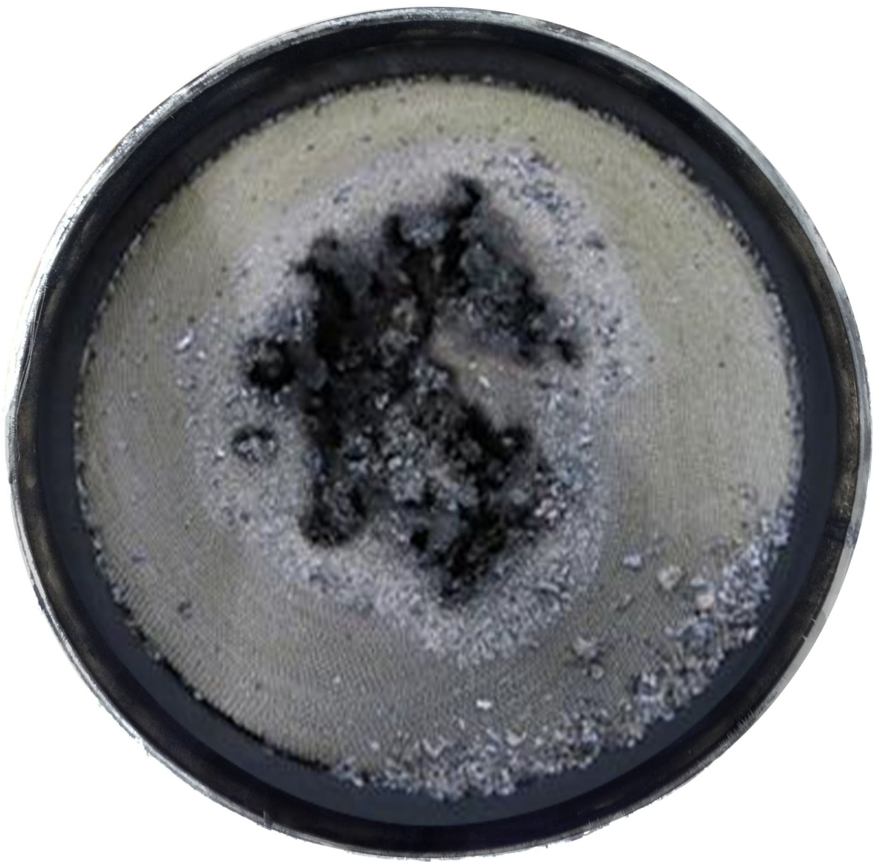
Figure 56 Diesel Oxidation Catalyst (DOC) - Melted.
