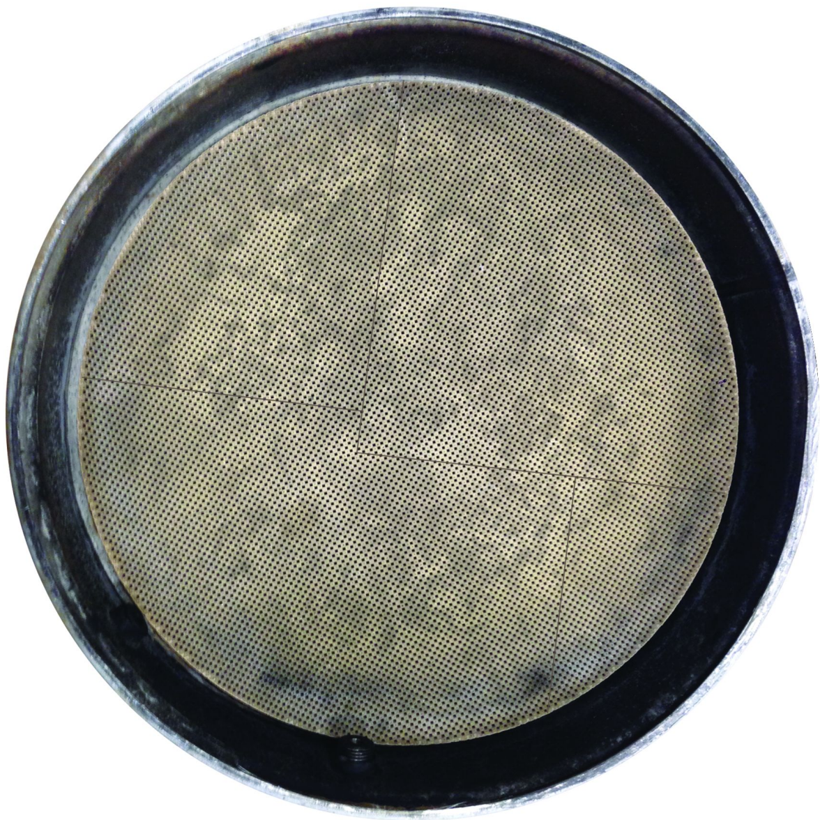
Figure 50 Diesel Particulate Filter (DPF) - Cracked, but Reusable.
