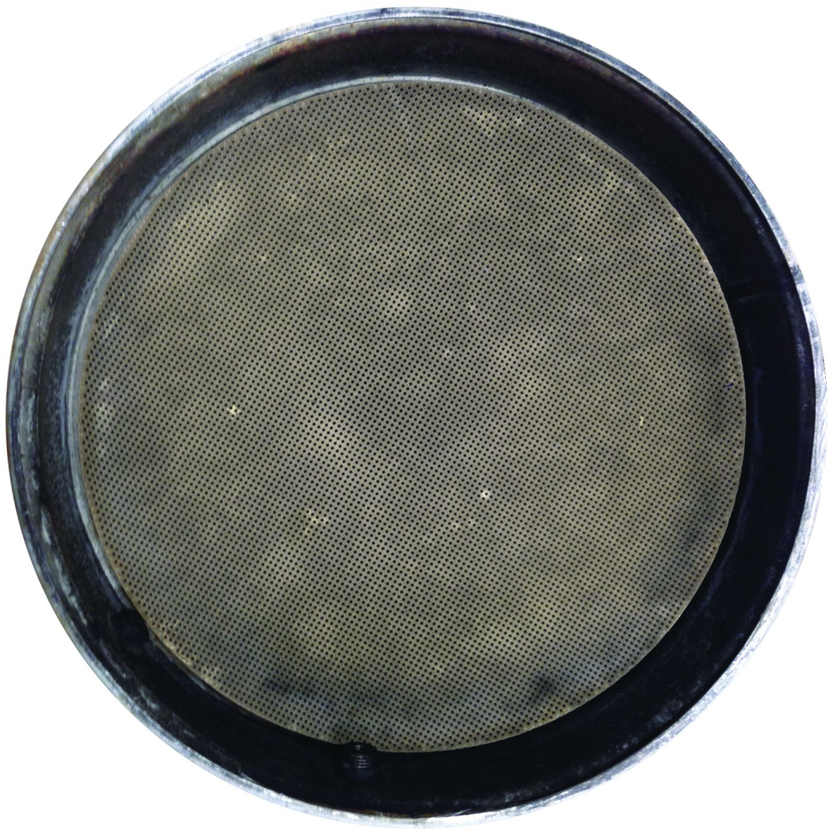
Figure 46 Diesel Particulate Filter (DPF) Inlet - Clean.
