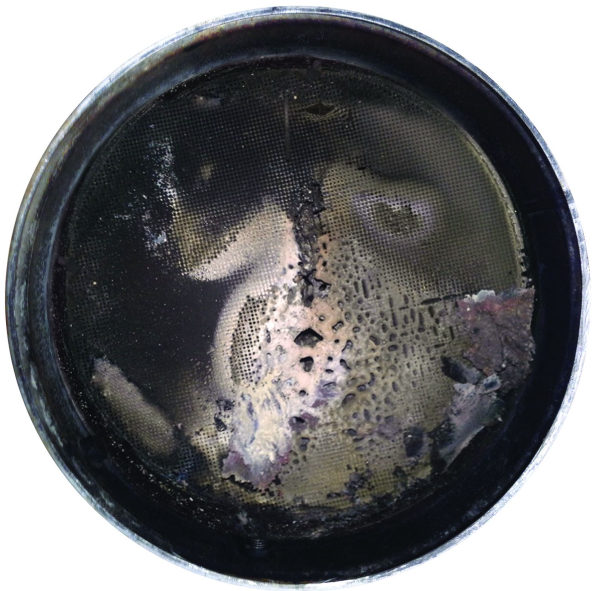
Figure 49 Diesel Particulate Filter (DPF) - Melted.
