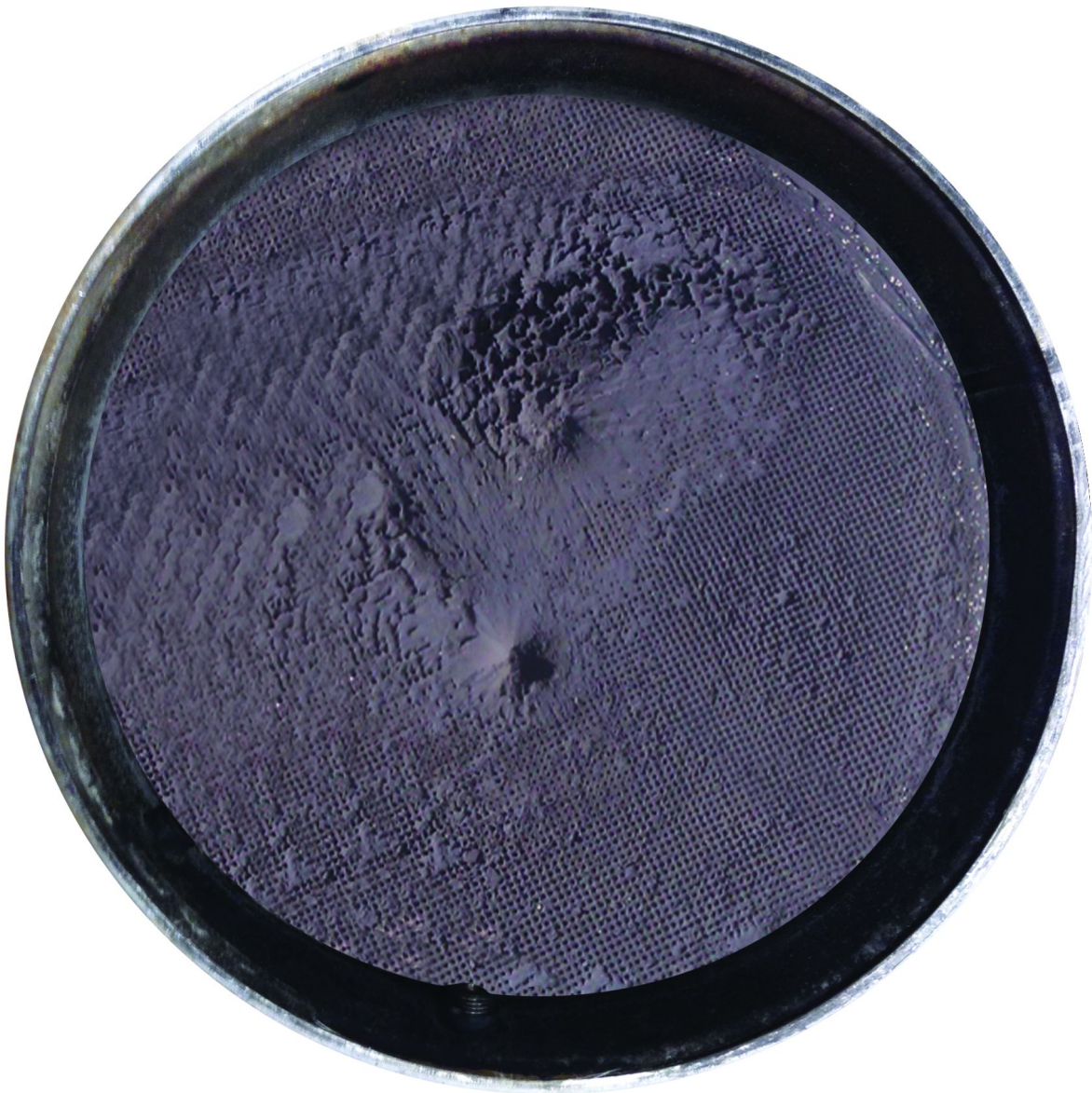
Figure 48 Diesel Particulate Filter (DPF) Inlet - Face Plugged.
