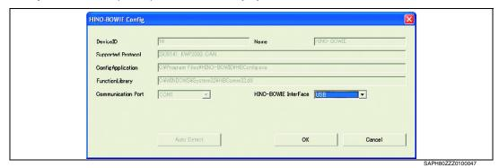
Fig. 1-30 Selecting USB Connection
