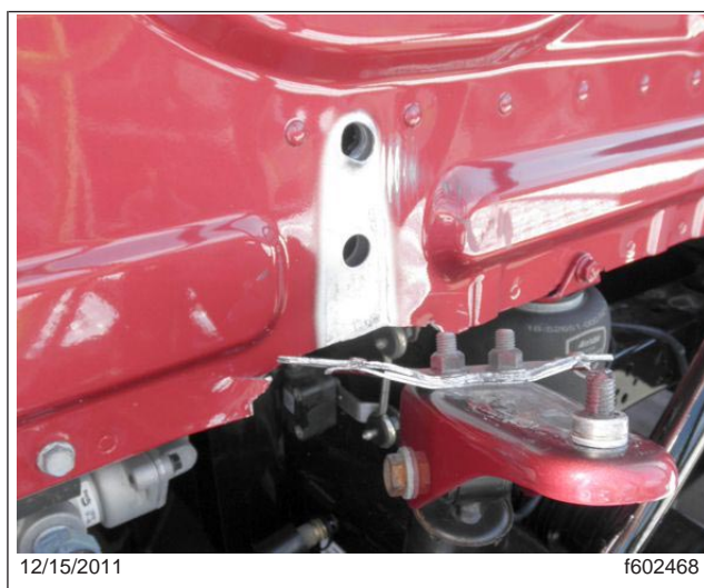
Fig. 1, Torn-Out Shock Mount Bracket, Back Wall of Cab
