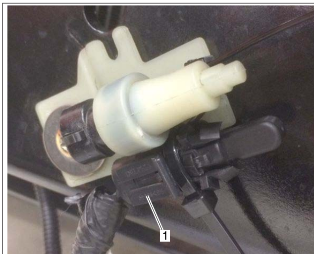
Fig. 2, New Ambient Air Temperature Sensor, Installed
