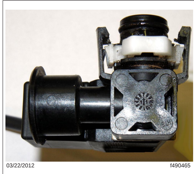
Fig. 2, 10-Watt Solenoid Valve ( 13.5\pm0.7\ \Omega )
