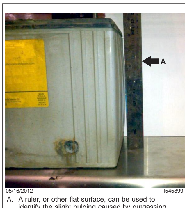
Fig. 2, Bulged 8A31 Battery Case
