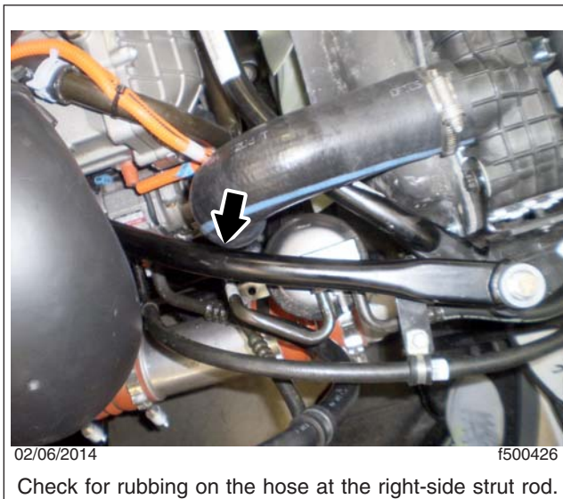
Fig. 1, Hose Rubbing Area, DD13 Engines
