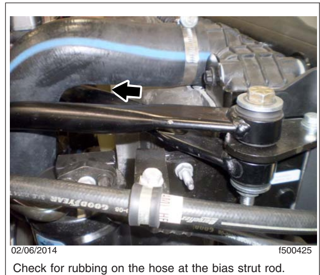
Fig. 2, Hose Rubbing Area, Cummins ISX Engines
