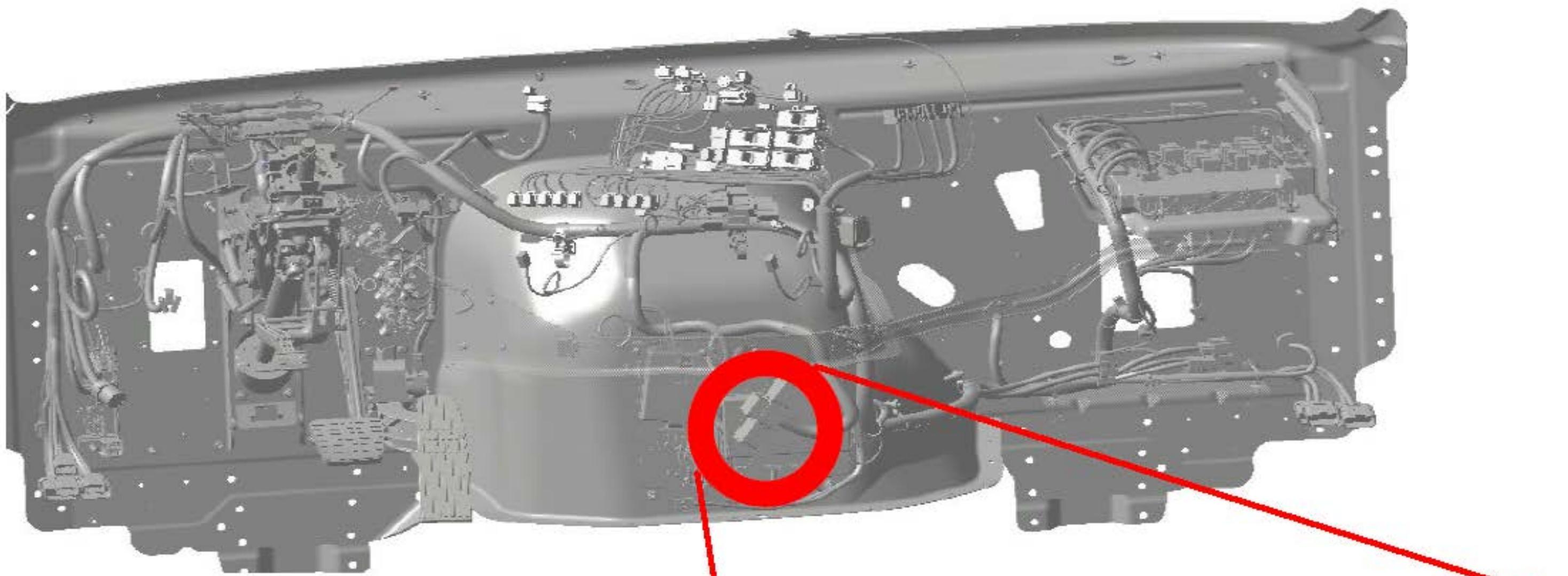
Location the PTCAN Share point and Cascadia SAM module CAN link, Star point inside of the cab under the dash.
