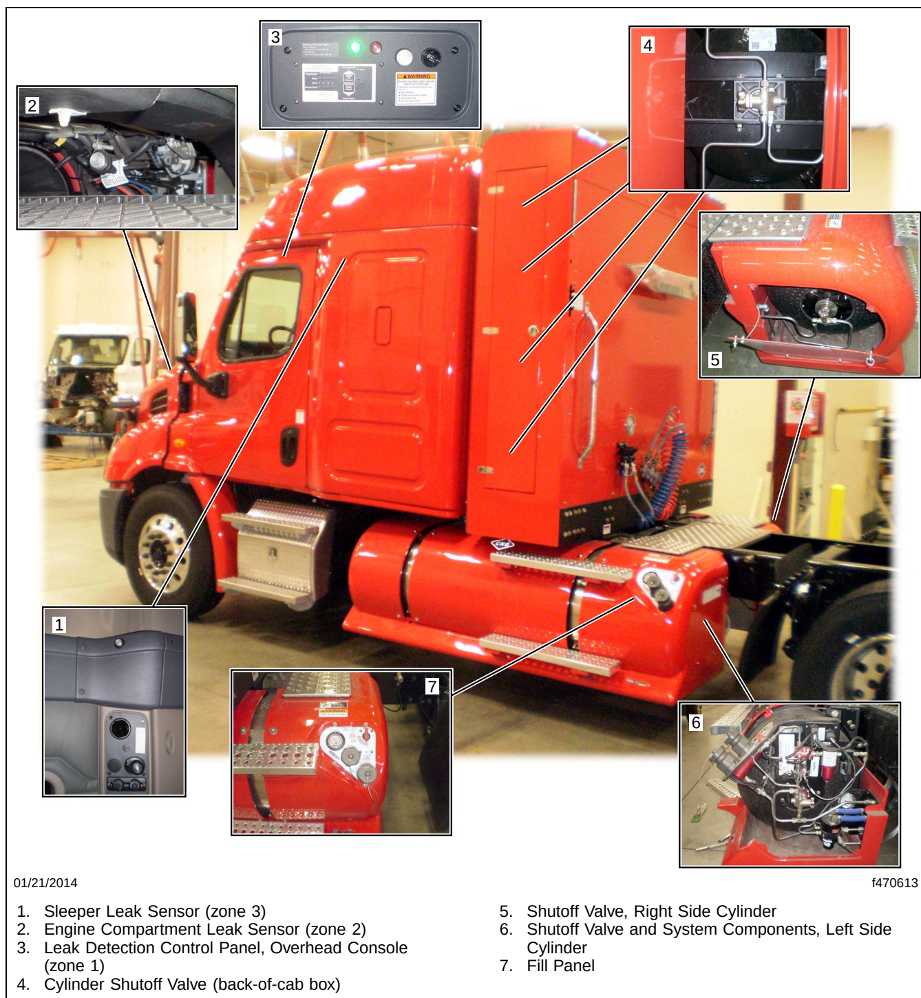
Fig. 1, Natural Gas Detection System Components
