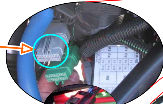
Transmission Interfaces. (Grey Plug) (Plugs may also be frame located (Module , 34C)
