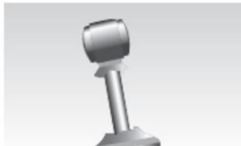
Damaged dust cover and/or shock body
