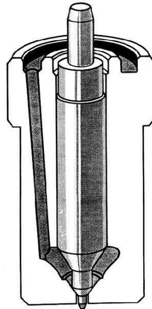
Fig. 15 - Schematic of fuel injector and nozzle holder
