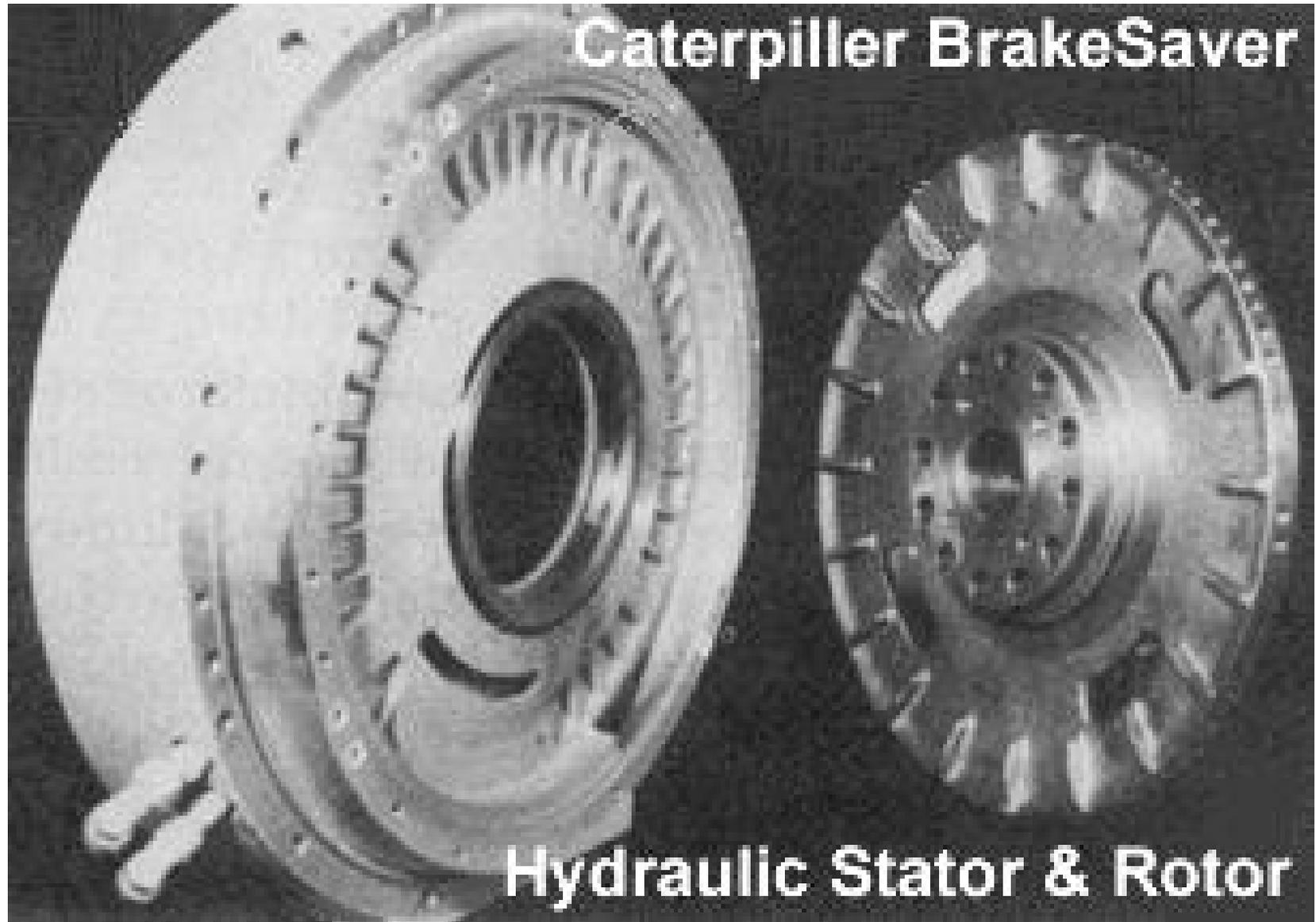
Hydraulic Stator & Rotor
