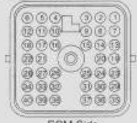
NOTE A: If the ECM Serial No. ends in "CA" the Vehicle Speed signal routes through the ECM pins 4, 10, 39, and 40. If the ECM Serial No. ends in "CG" or "CJ", pins 4 and 39 are used for Timing Calibration only, pins 10 and 40 are unused.
