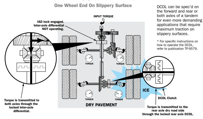
Forward axle can develop high torque due to dry pavement. Rear axle can develop high torque on dry road side.
