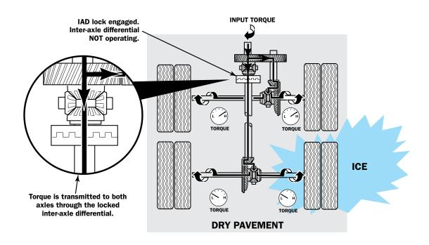
Forward axle can develop high torque due to dry pavement. Rear axle torque limited by wheel on slippery surface.
