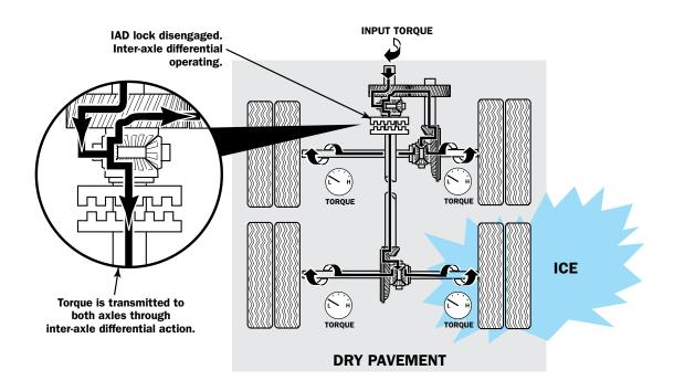
Torque to all wheels is limited by the wheel on the slippery surface.
