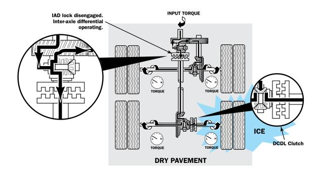
Torque to all wheels is limited by the wheel on the slippery surface.
