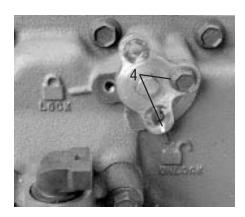
Rotate the Lock Cover counterclockwise until the indication notch lines up with the unlock symbol, and secure the cover in position by inserting one of the capscrews into the rightside hole.
