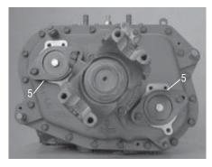
5. Remove Auxiliary Countershaft Bearing Covers, shims and gaskets. Install RR1002TR Auxiliary Countershaft Support Straps.
