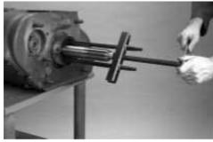
5. Install the RR1023TR Input Shaft Bearing Puller and remove the Input Bearing.
