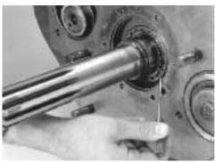
7. Pull the Input Shaft forward and out of the Drive Gear.
