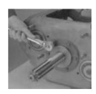
2. If present, remove and discard the rubber seal ring on the Input Shaft. The ring is used only to seal the Transmission during shipment.
