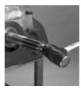
4. Use a RR1019TR Hand Maul to drive the Input Shaft toward the case rear as far as possible. Pull the Input Shaft forward.
