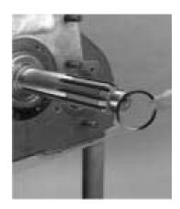
3. From the Input Shaft groove, remove the bearing retaining snap ring.
