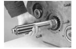
8. Inspect the bushing in the Input Shaft pocket, replace if damaged.
