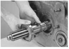
6. Remove the Drive Gear Internal Snap Ring.
