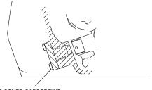
OIL PUMP COVER CAPSCREWS 12-14 N.m [9-10 lb. ft.] M6x1 THREAD
