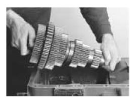
2. Place the lower, 47-tooth PTO Gear Countershaft, into the Main Case with the shaft seated in the Lower Countershaft Case bores.
