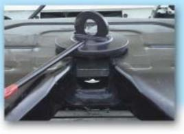
Verify that the pull handle is in the fully locked position (within 1" of the fifth wheel skirt).
