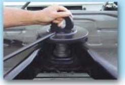
Carefully push the kingpin in until the locking mechanism is activated. Keep your hands and arms out of the fifth wheel throat.
