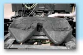
Grease the mount brackets (4 zerks). Lift the top plate up with a pry bar to ensure grease gets to the top of the brackets.
