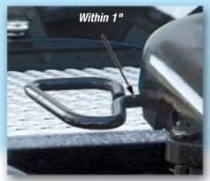
Note: See the Fontaine Instruction Handbook (LT001) for complete details. Check the travel of the wedge stop rod with thumb pressure. You should have 1/4" movement. If less, turn wedge stop rod counter clockwise; if more, turn clockwise.
