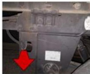
Unlock the locking pins axles
