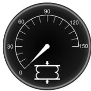
Although optional, the suspension air pressure dial is very useful when used judiciously. The greater the load on the suspension, the greater the pressure in the suspension. The driver must make connections between the dial reading and the scale reading when they weigh their truck.
