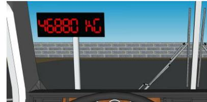
NB. The brakes must be released in each weighing session, otherwise the results could be inaccurate.
