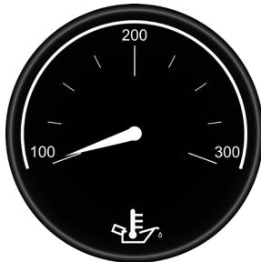
Oil temperature should be maintained between 200 °F and 260 °F
