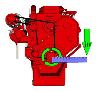
The power of an engine is calculated in the same way. In the second example, the engine develops a rotational force of **1650 lb/ft**. Typically, truck engines develop between 1250 and 1850 lb/ft of torque.
