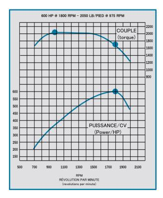
In this second example, the 16L engine develops **2050 lb/ft of torque @ 975 RPM.**
