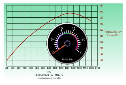
In the example on the left, the engine is developing **485 HP @ 1650 RPM**.
