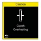
When these indicators come on in the instrument panel, it means that the clutch is <u>overheating</u>, and the clutch may stop working. A protection system can then momentarily disengage the clutch, to allow it to cool. It will therefore be impossible, under these conditions, to move the vehicle.
