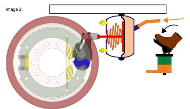
The compressed air puts pressure on the membrane (diaphragm) contained in the brake actuator (booster)
