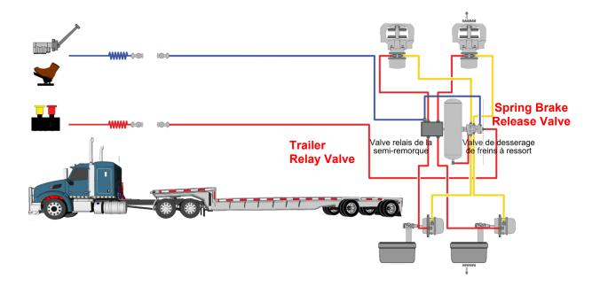
When the red button is pushed, the semi-trailer is supplied with air. When there is sufficient pressure, the parking brakes are released. The air supply to the semi-trailer is provided by the red hose.
