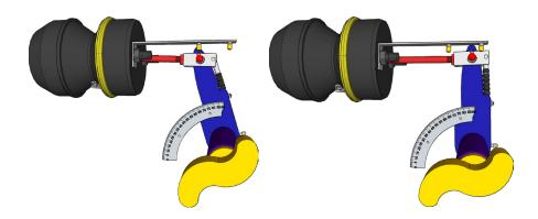
Slack adjustment procedure for vehicles equipped with brake drums:
