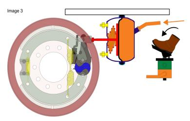
The higher the air pressure, the more load the diaphragm exerts on the push rod, which in turn exerts pressure on the adjustable lever (slack adjuster). The adjustable lever (slack adjuster) imposes a rotational force on the "S" Camshaft. It is the action of this rotation that acts on the brake shoes and causes the brakes to apply.
