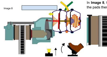
In Image 8, the parking brake is applied; the pads then clamp the disc.
