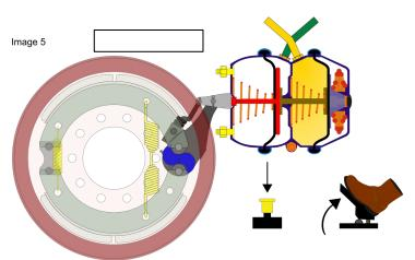
By pushing the yellow button, air enters the cylinder and pushes on the diaphragm, compressing the parking brake spring and the brakes become released.
