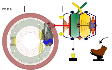
This image shows that the parking brake spring is compressed by the air pressure coming from the parking brakes yellow button and the service brake is applied by the air pressure coming from the brake pedal.
