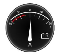
An ammeter (optional dial) measures the intensity of an electric current. Its normal reading is slightly above zero. If there is a strong current demand, the reading will increase on the positive side. On the other hand, if the alternator stops working, the reading will go to the negative side.
