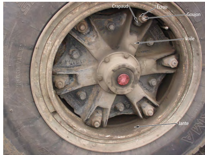
FIGURE 45 | Roue moulée ( spoke wheel )
