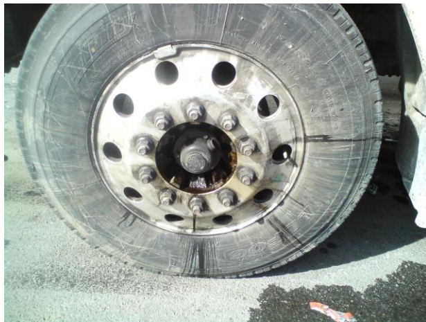
Examples of defects caused by seal leakage.
