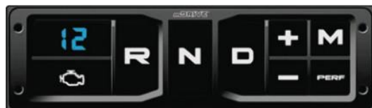
Mack M-Drive control switch found on the dashboard.
