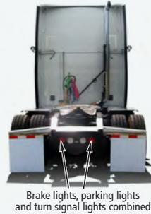
**FIGURE 31** | Rear lights of a semi-trailer
