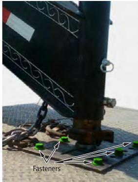
FIGURE 17 | Ball and hitch coupling device
