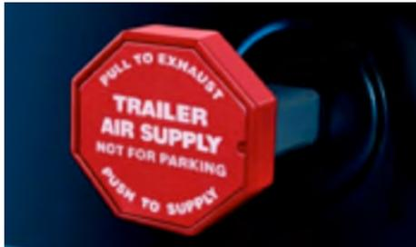
FIGURE 65 | Parking brake air supply control
