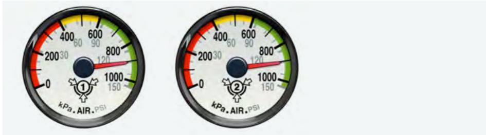
The compressed air pressure gauges indicate the air pressure in the service tanks of the bus, truck or tractor. Because the service brake system has two independent circuits, there are two gauges on the dashboard, that is, one for each circuit: the primary and secondary circuits. Some vehicles are equipped with a single gauge with two needles, one for each circuit.
