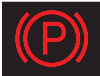
FIGURE 61 | Service brake warning light
