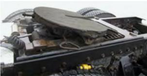
FIGURE 2 | Coupling plate and kingpin
