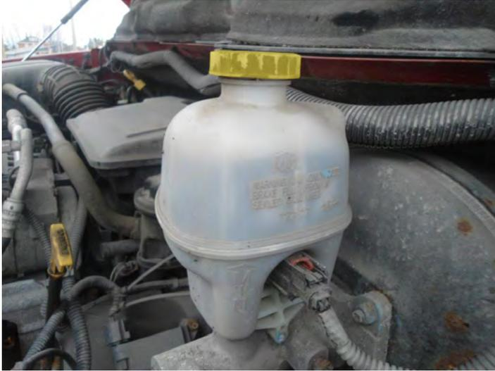
**FIGURE 57** | Master cylinder reservoir of a school bus
