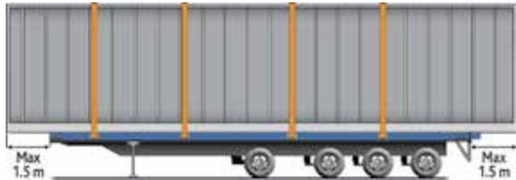
In all cases, the container must be secured against moving sideways, lengthwise or vertically in accordance with:
