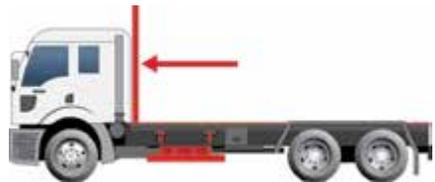
The **width** of the front-end structure of a vehicle must not be narrower than the narrower of the following two measures:
