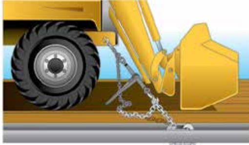
The accessory equipment on a heavy vehicle (e.g. hydraulic shovels) must be completely lowered and secured to the vehicle, unless the equipment:
