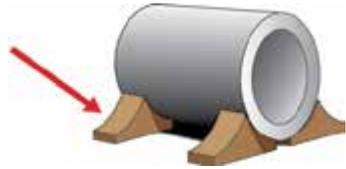
Each pipe in the front half of the group of pipes, including the middle one where there is an odd number, must be secured by **at least one (1) tiedown**:
