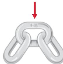
– For example, a chain that is compliant with the standard of the National Association of Chain Manufacturers has a WLL equivalent to that standard, according to the grade and size indicated on the chain.
