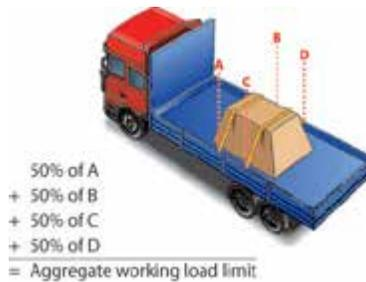
When a WLL is identified by a label referring to the numerical value of the WLL (e.g. 3 000 kg), this label is deemed to be the WLL of the device or component.
